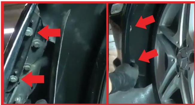
21) Move to the corner and replace the (2) 10mm bolts that secure the bumper to the fender and the (2) 10mm bolts that secure the fender liner to the bumper.
