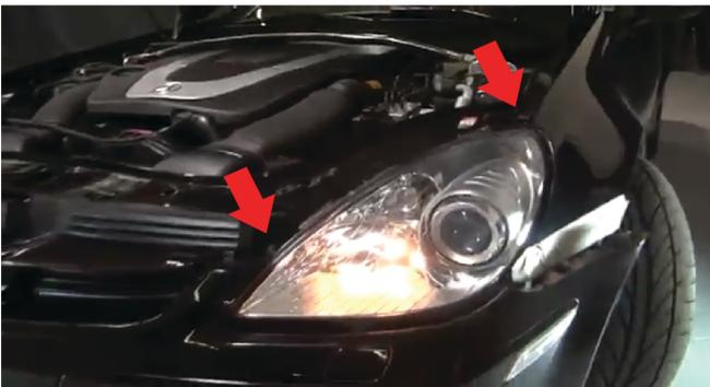
7) Top side you will need to remove the (2) 10mm bolts on the head light to loosen it from the frame. The locations are shown above.
