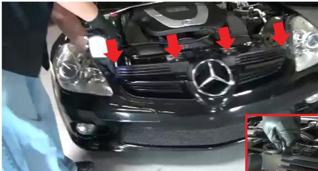
1) Open your hood and locate the (4) 10mm bolts. Two securing the bumper and two on the grill, use your 10mm socket for the outer (2) 10mm bolts and use your 10mm wrench to loosen the (2) center 10mm bolts, unthread them with your fingers after.
