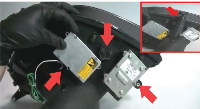
15) Next, replace the (2) ballasts and nozzle clip down first. Once you have crewed these all back into place first then replace the washer nozzle onto the clip and last screw to hold it into place.
