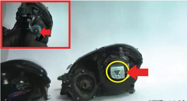
13) The next step is to Remove the HID box and bulb from the old head light. Simply twist the HID box counter-clockwise to remove and expose the bulb. Unclip the bulb by removing pinching the pins together. Note: do not touch the bulb by its glass, oils from your fingers can cause damage when later plugged in.
