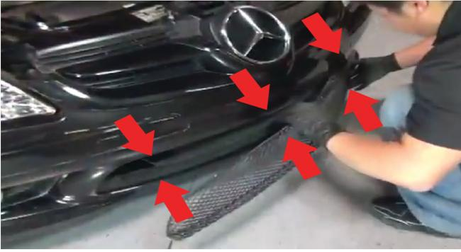
5) Next, the grill must be removed to expose (2) 10mm bolts that will release the bumper from the frame. Using the flat head-driver locate the tabs and gently push down on them popping out the grill (be sure not to be on the grill).
