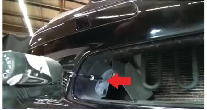
6) Next, once the grill has been removed, use the 10mm socket, remove the (2) bolts securing the bumper down. Set these aside with the bumper so that they are together.
