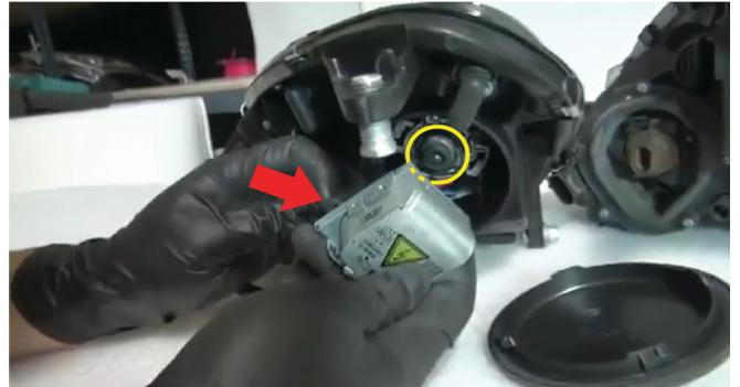
14) Now we will be reinstalling the HID bulb and HID box into the new head light. Place the HID bulb into the new housing and use the pins to secure it to the socket. Next, plug the connector into the HID box, secure the box onto the back of the bulb by twisting it clockwise into place. Replace the backing securely to close the head light.
