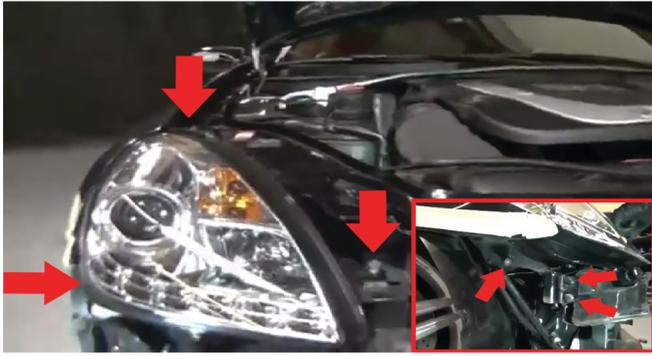
17) Reinstall the (5) 10mm bolts that secure the head light to the frame. There will be (2) on the top and (3) on the side as shown.
