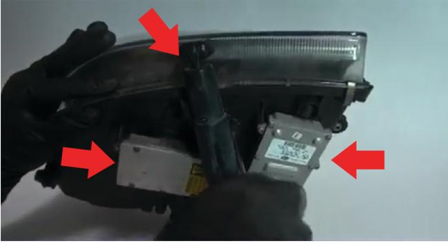
11) Now that you have the head light removed there will be several items needing to be transferred to the new head light. First, on the underside you will need to remove (2) ballast and (1) washer nozzle. Use the Phillips screw driver, unscrew the nozzle from the top first and pop it from its clips to expose the other two screws beneath it. Next remove the ballasts.
