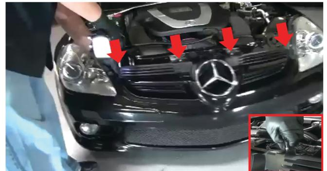
22) Lastly, bolt down the (4) 10mm bolts securing the grill section. Note: if you installed the two center bolts in step 19 you will only have the two other grill/ bumper bolts to install. Be sure that all bolts are secured tightly and you have not completed the installation of your new Spyder head lights on your 05-10 Mercedes Benz R171 SLK with HID.
